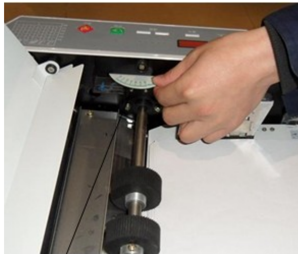
Pressure adjusting dial↵ for paper standing↵
