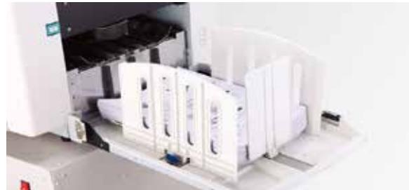
Normally 1000 sheets paper-receiving capacity, even can reach 1200 (60g/m<sup>2</sup>)sheets. Paper feeding tray can heap 1000 sheets at once during high-speed printing.
