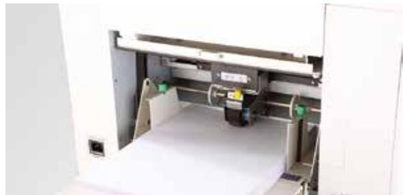
Innovative design of paper feeding by double rollers which is much stable. Simultaneously feed paper to guarantee one page input only once time.
