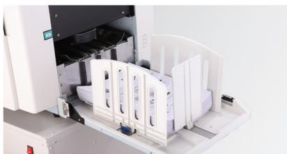
Master eject capacity is easy for 40 sheets.
